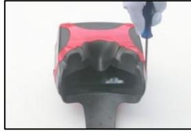
2. Lift off the bottom part of the casing. Display, control panel and lens remain in the top part.
