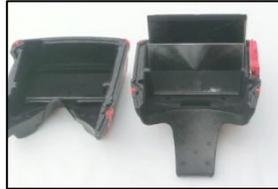
3. Remove the preinstalled Fresnel lens. Clean the display.
