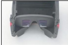
5. Turn around the bottom part and close the casing. Check that the HPRO is clamped in correct position and parallel to the display.
